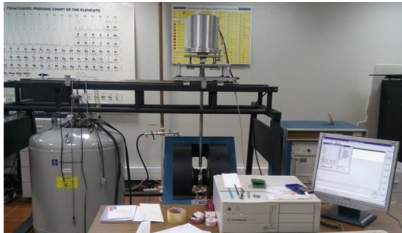
Figure 1. Vibrating sample magnetometer (VSM) to be used for magnetic measurements.
